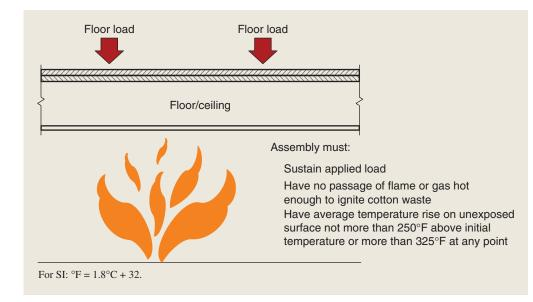
Figure 703-2 Floor assembly fire test.
