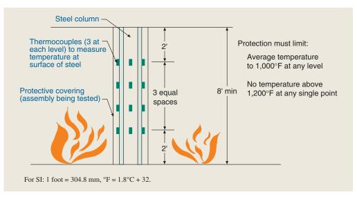
Figure 703-5 Alternative fire test of steel column protection.
