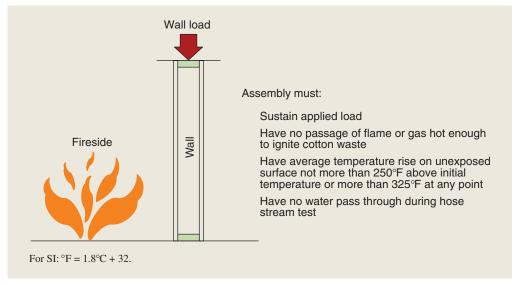
Figure 703-3 Conditions of acceptance wall fire test.
