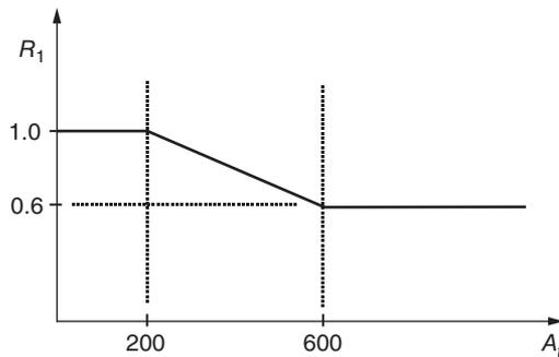
**FIGURE 3.2** Graph showing permitted live-load reduction for roofs. (Source: Section 1607.11.2 of the 2015 IBC.)
