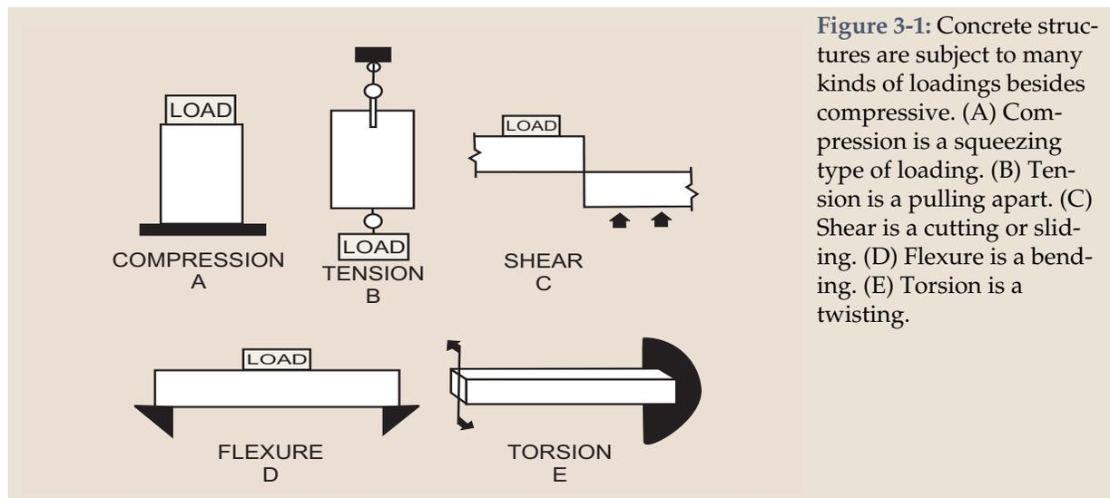
**Figure 3-1:** Concrete structures are subject to many kinds of loadings besides compressive. (A) Compression is a squeezing type of loading. (B) Tension is a pulling apart. (C) Shear is a cutting or sliding. (D) Flexure is a bending. (E) Torsion is a twisting.
