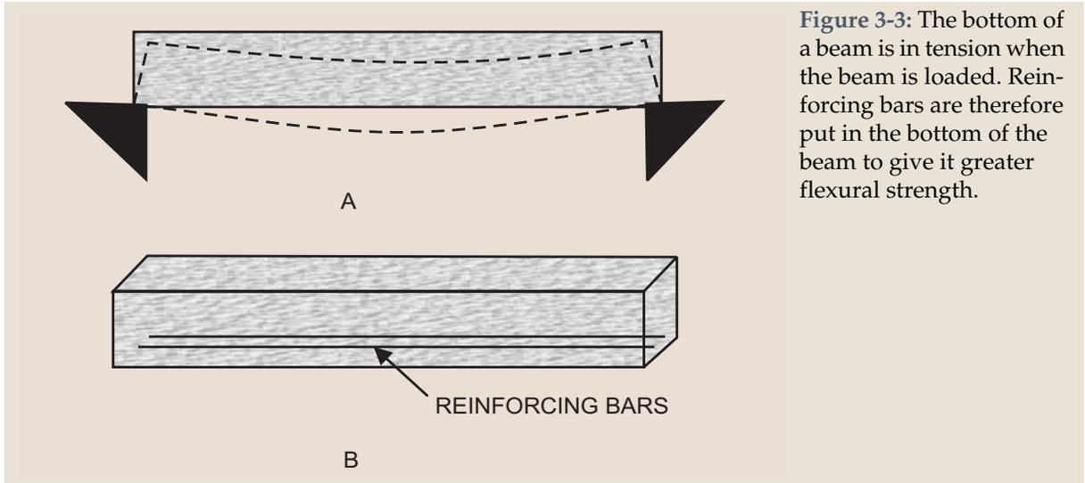
**Figure 3-3:** The bottom of a beam is in tension when the beam is loaded. Reinforcing bars are therefore put in the bottom of the beam to give it greater flexural strength.
