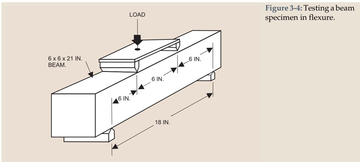
**Figure 3-4:** Testing a beam specimen in flexure.
