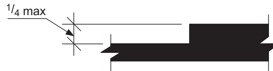
FIGURE 303.2—VERTICAL CHANGE IN LEVEL
