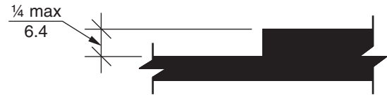
FIGURE 303.2 VERTICAL CHANGE IN LEVEL
