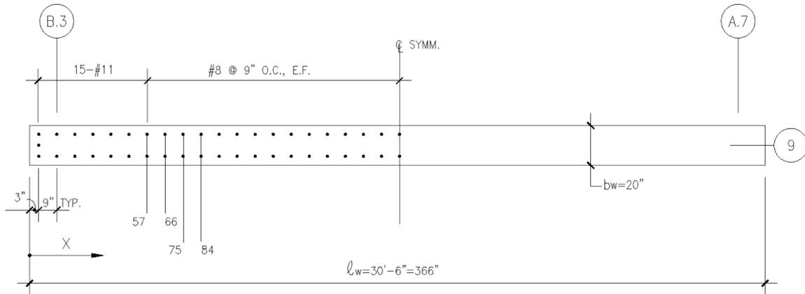
Figure 1-3. Layout of vertical reinforcement at wall base
