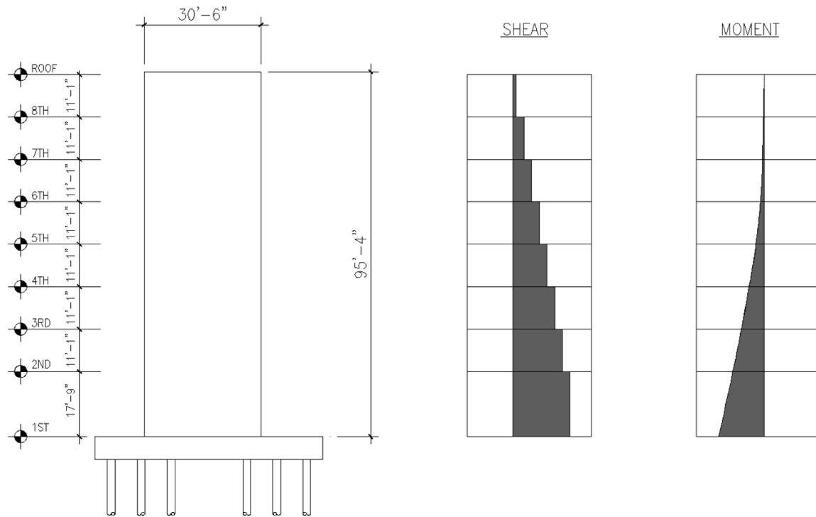
Figure 1-2. Wall elevation, shear, and moment diagram
