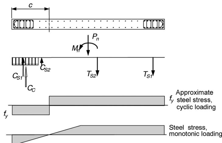
Figure 1-4. Steel stress and neutral axis depth
