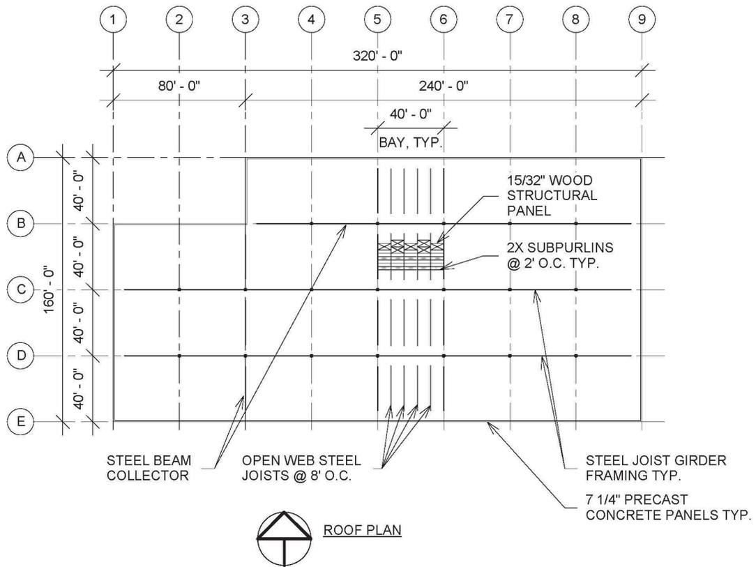
Figure 2-2. Example's roof plan
