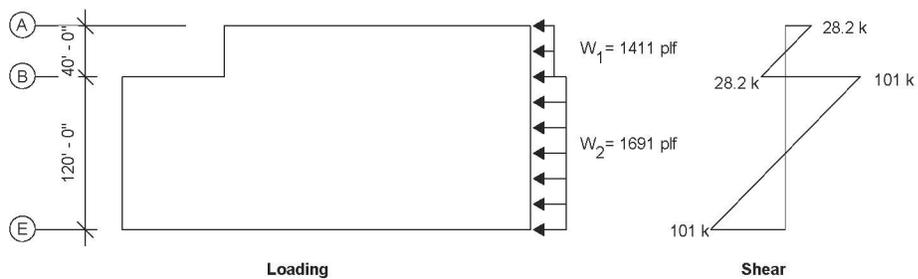
Figure 2-4. East-west diaphragm loading
