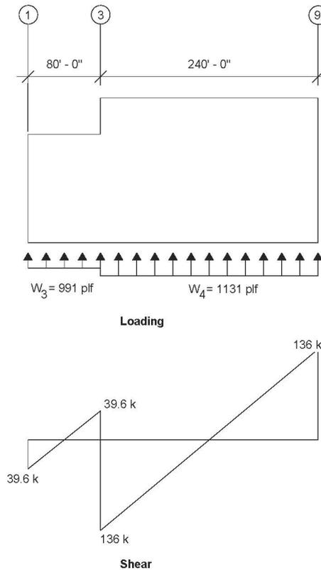
Figure 2-5. North-south diaphragm loading
