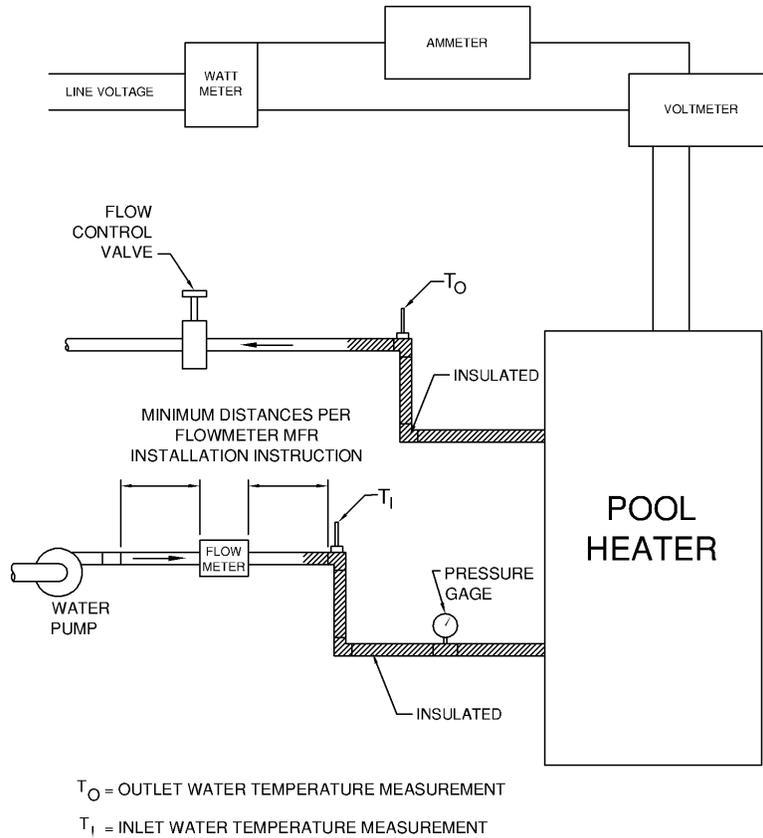
Figure 1a Plumbing layout and location of water temperature measurements (heat pump pool heaters).
