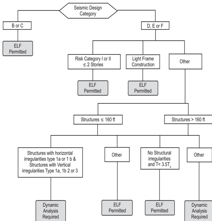
For buildings in SDC D, E or F, the trigger for Dynamic Analysis (Modal Response Spectrum Analysis or Seismic Response History Procedures) is based on the height of the building—buildings that are less than 160 feet in height and have horizontal torsional irregularities of Type 1a or 1b and vertical irregularity Type 1a or 1b, 2 or 3, Dynamic Analysis is required.
