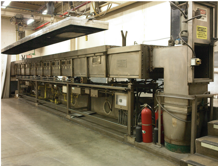
The Steiner Tunnel Test referred to in ASTM E84 measures a material's flame spread and smoke-developed indexes. (Photo courtesy of Underwriters Laboratories, Northbrook, IL)
