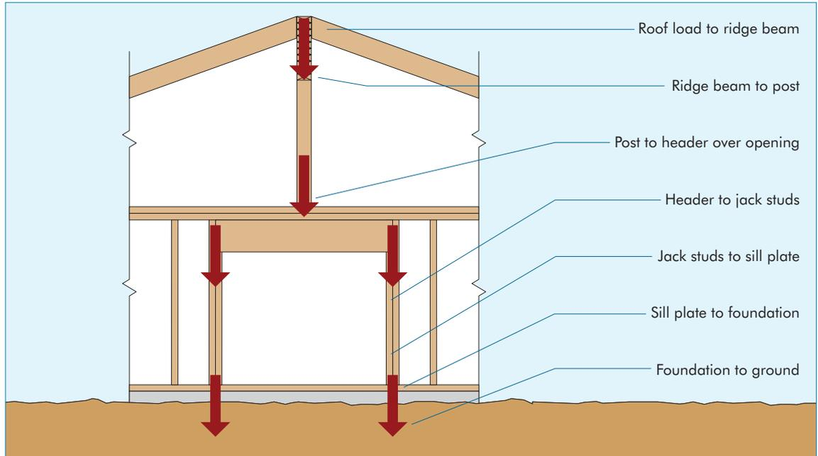
The upward load path is the same as the downward load path except the load is acting in the “up” direction. Upward (wind uplift) loads must be resisted by uplift straps and/or structural wall sheathing, connectors and anchors that keep the structure intact and attached to the foundation.
