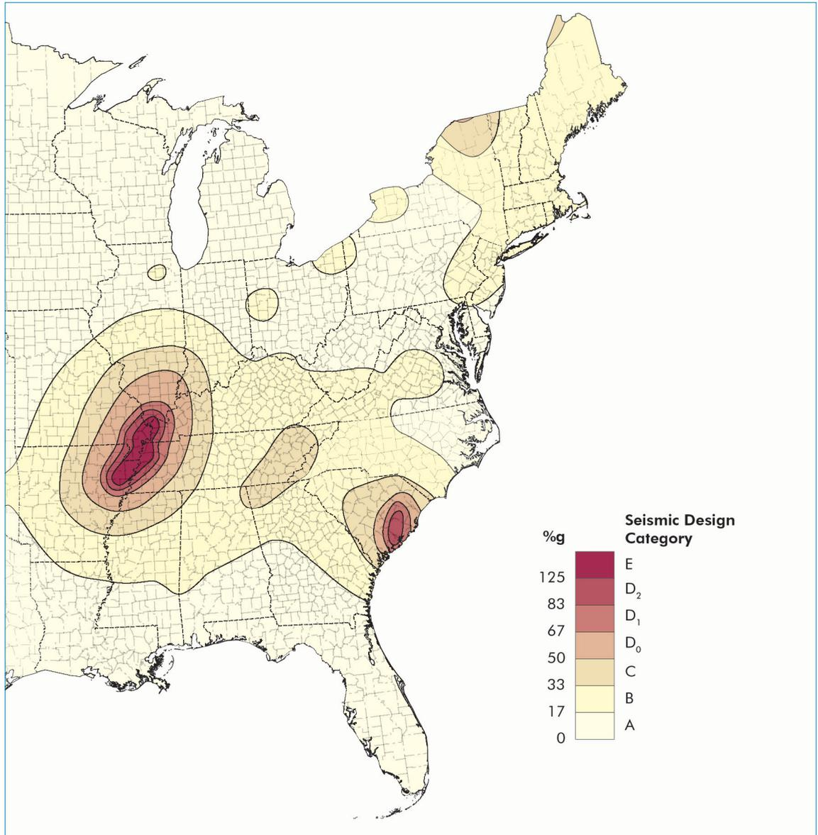
The use of Seismic Design Categories is a simplified means of determining the potential hazard of an earthquake in a region. For residential structures, these categories range from Seismic Design Category (SDC) A to E, with A being the lowest hazard and D<sub>2</sub> the highest covered by the IRC.
