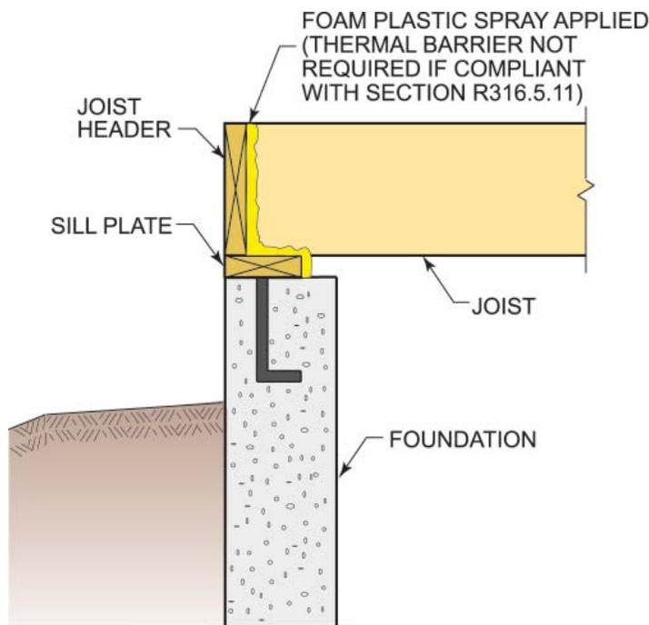
Foam plastic spray applied to sill plate and header
