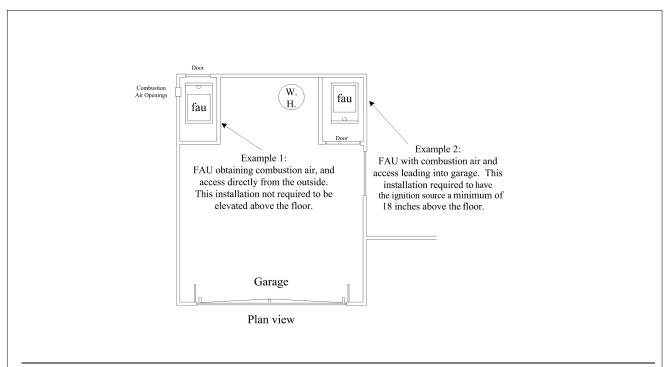
Water heaters that are listed as flammable vapor ignition resistant are exempt from the requirement to elevate the ignition source 18 inches above the floor and are permitted to be located in a garage at floor level without separation.
