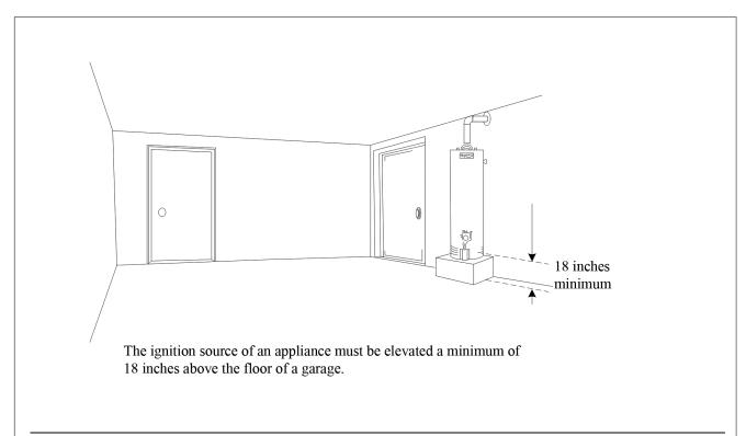
Examples of appliance ignition sources include the burners of a furnace, dryer or water heater; burner igniters or electrical relays; switches; contacts; and electrical motors, which can create a spark.
