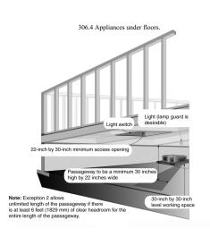
For both attic and under floor installations, a light fixture (luminaire) and a receptacle outlet are required at the appliance location for use during the service or repair of the equipment. The switch controlling the light fixture must be located at the entry to the passageway.
