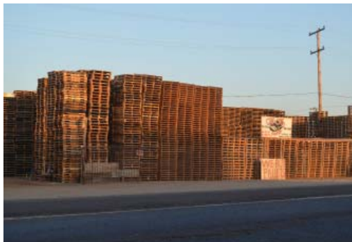
FIGURE 3-3 Outdoor storage of idle pallets can pose a significant fire exposure.
