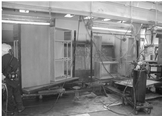
Figure 3-3: Open-Face Spray Booth
