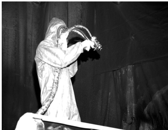
Figure 3-2: Spray Application of a Bed Liner
