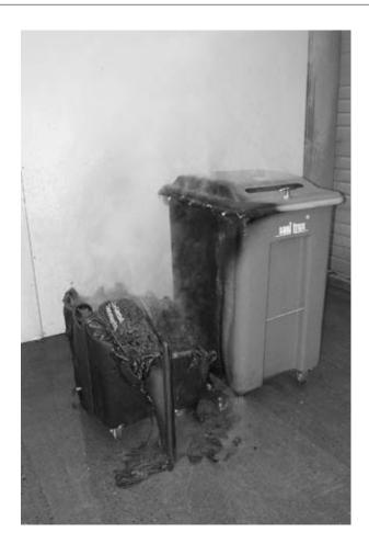
The trash container on the right passed the ASTM E1354 fire test and did not contribute to the fire.
