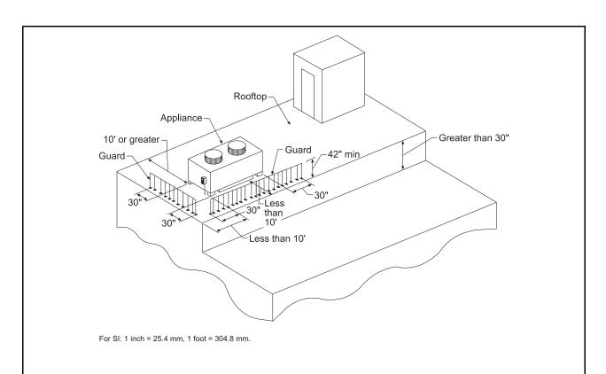
Permanent fall arrest/restraint connector devices are considered equivalent to guards for worker safety on a roof. Service personnel in safety harnesses can connect to the restraint anchors to prevent injury from falls.
