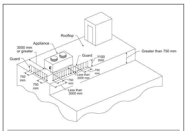
Permanent fall arrest/restraint connector devices are considered equivalent to guards for worker safety on a roof. Service personnel in safety harnesses can connect to the restraint anchors to prevent injury from falls.
