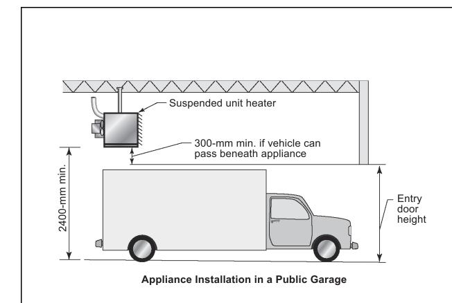
Where another means of protection is provided to eliminate the potential for vehicle impact, such as a vehicle barrier, the appliance need not be located at the minimum prescribed height. It is, however, necessary that the appliance comply with Section 304.3 (elevation of ignition source) and NFPA 30A (Code for Motor Fuel-dispensing Facilities and Repair Garages).
