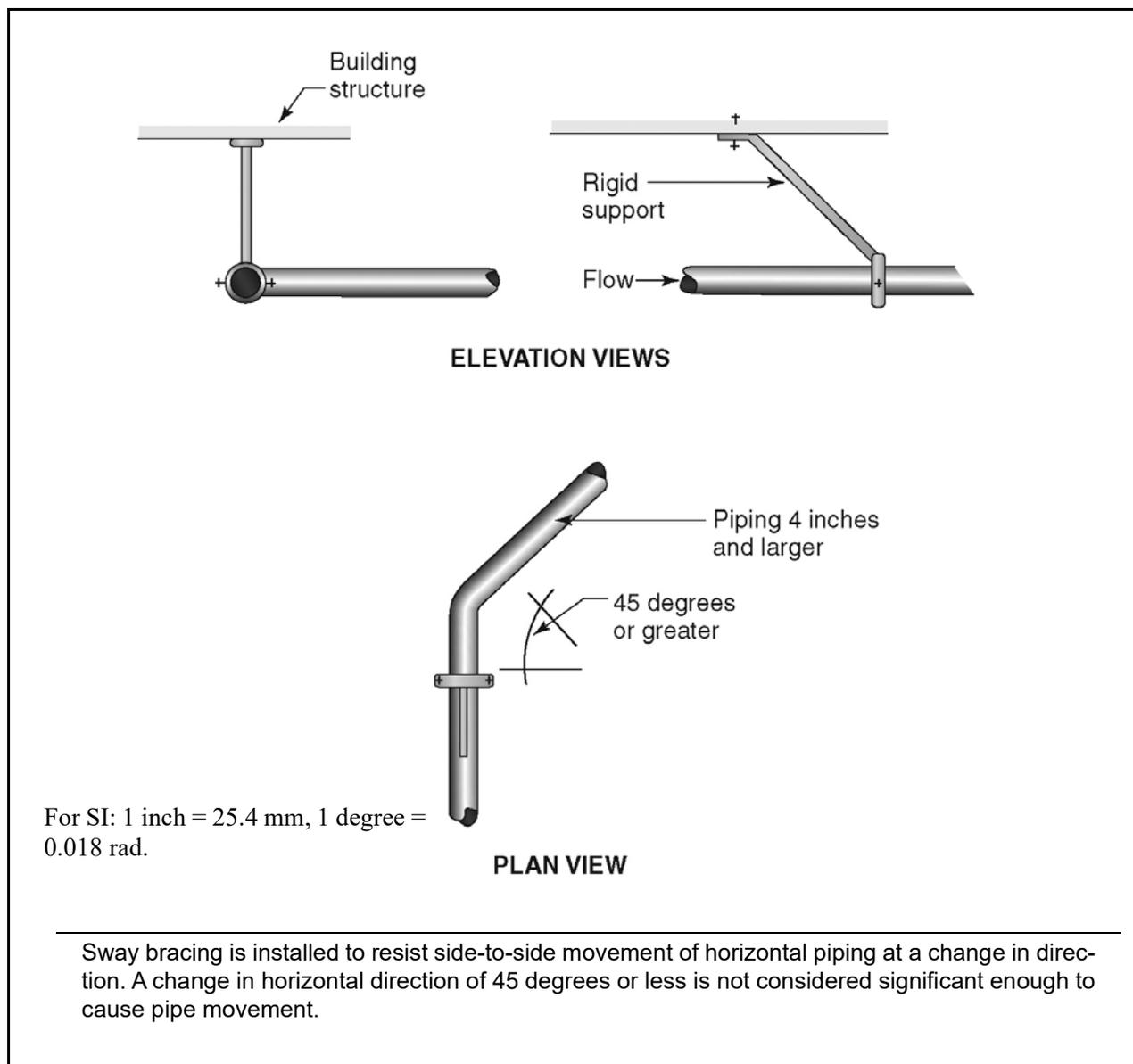
**Code Text:** *Anchorage shall be provided to restrain drainage piping from axial movement. For pipe sizes greater than 4 inches (102 mm), restraints shall be provided for drain pipes at all changes in direction and at all changes in diameter greater than two pipe sizes. Braces, blocks, rodding and other suitable methods as specified by the coupling manufacturer shall be utilized.*
