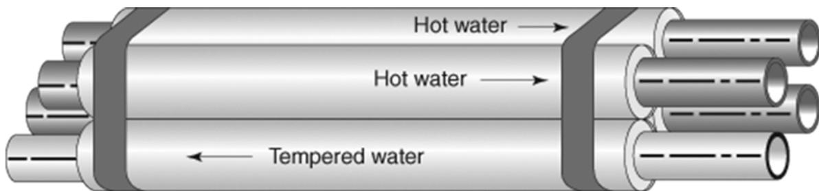
To prevent thermal transfer, the code requires each hot water pipe to be insulated when hot water piping is bundled with other piping. Bundles of PEX piping typically are held together loosely with plastic ties to allow for expansion and contraction of the individual pipes.
