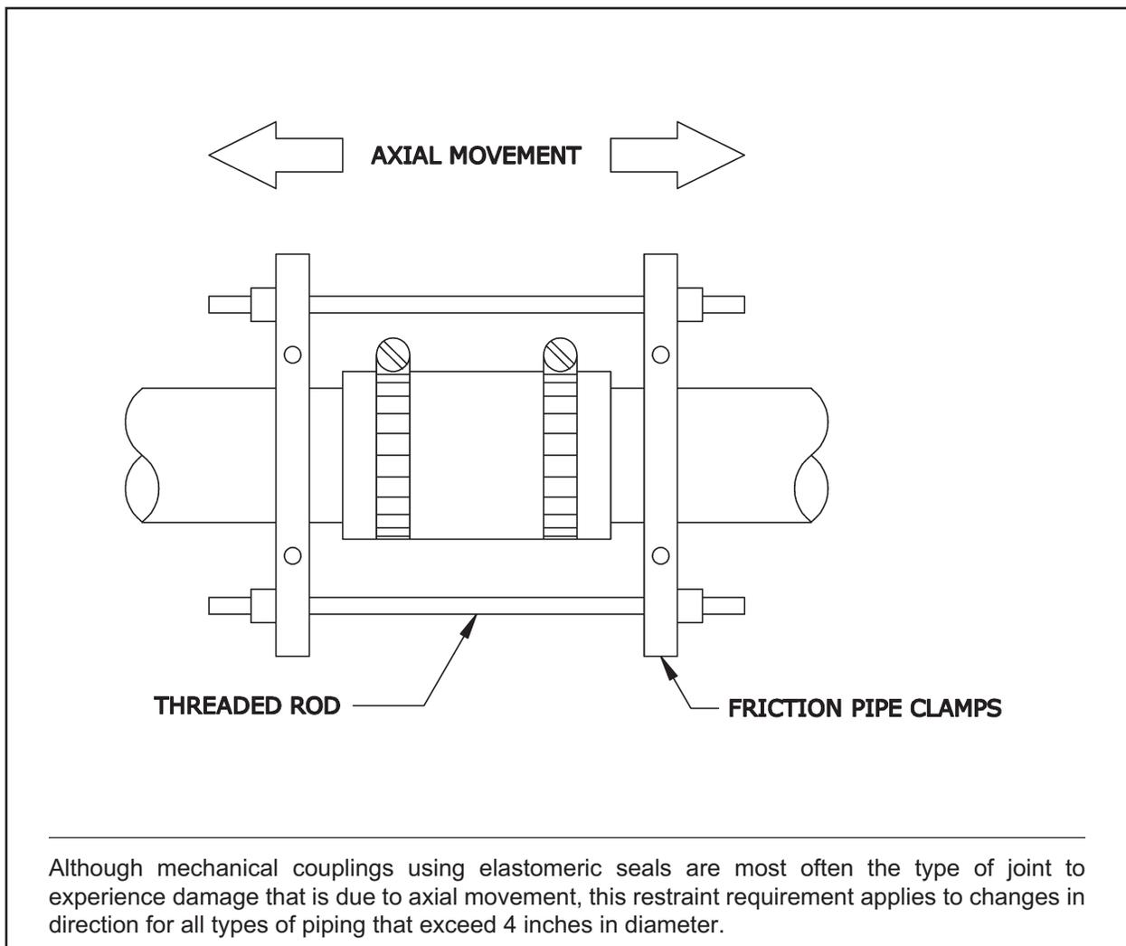
**Code Text:** *Piping bundles for manifold systems shall be supported in accordance with Table 308.5. Support at changes in direction shall be in accordance with the manufacturer's instructions. Where hot water piping is bundled with cold or hot water piping, each hot water pipe shall be insulated.*
