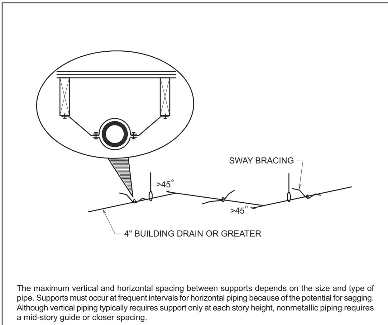
**Code Text:** *Anchorage shall be provided to restrain drainage piping from axial movement. For pipe sizes greater than 4 inches (102 mm), restraints shall be provided for drain pipes at all changes in direction and at all changes in diameter greater than two pipe sizes. Braces, blocks, rodding and other suitable methods as specified by the coupling manufacturer shall be utilized.*
