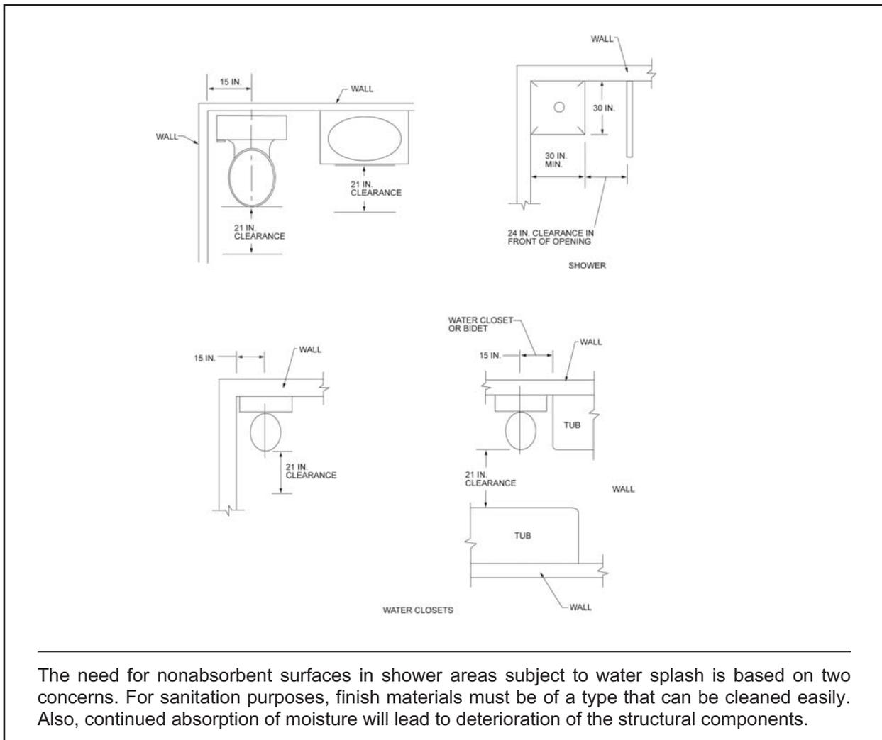
The need for nonabsorbent surfaces in shower areas subject to water splash is based on two concerns. For sanitation purposes, finish materials must be of a type that can be cleaned easily. Also, continued absorption of moisture will lead to deterioration of the structural components.
