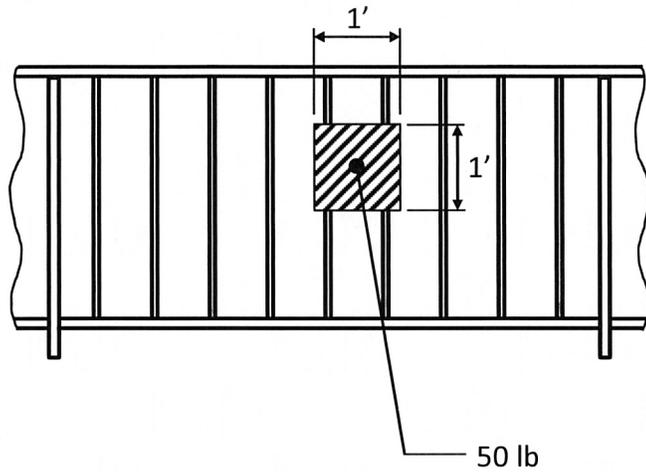
The concentrated load in load condition 1 is meant to simulate the maximum anticipated load from a person grabbing or falling into the handrail or guard while the line load in load condition 2 is the maximum anticipated load on a handrail or guard from use by a crowd of people on a stairway. These loads can occur in any direction, as shown in Figure 3.1, and need not be applied concurrently.
