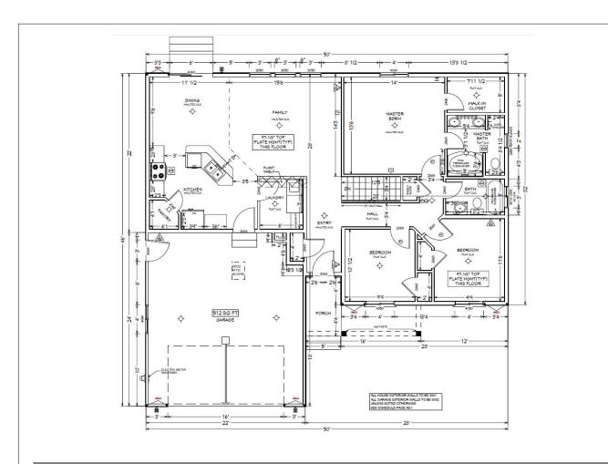
Basic projects such as room additions may also show electrical receptacles, lights and switches, plumbing lines and heat ducts on the floor plan instead of on separate drawings for each type of work. Furniture and other movable items do not typically need to be shown on a floor plan.
