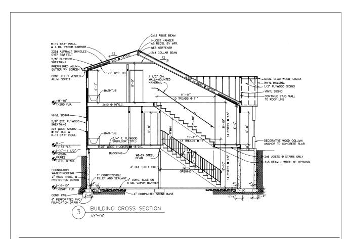
Section drawings are important because they show the builder, plans examiner and inspector in detail how certain aspects of the building will be connected or framed in. They also show various dimensions pertaining to window and door heights as well as ceiling heights.
