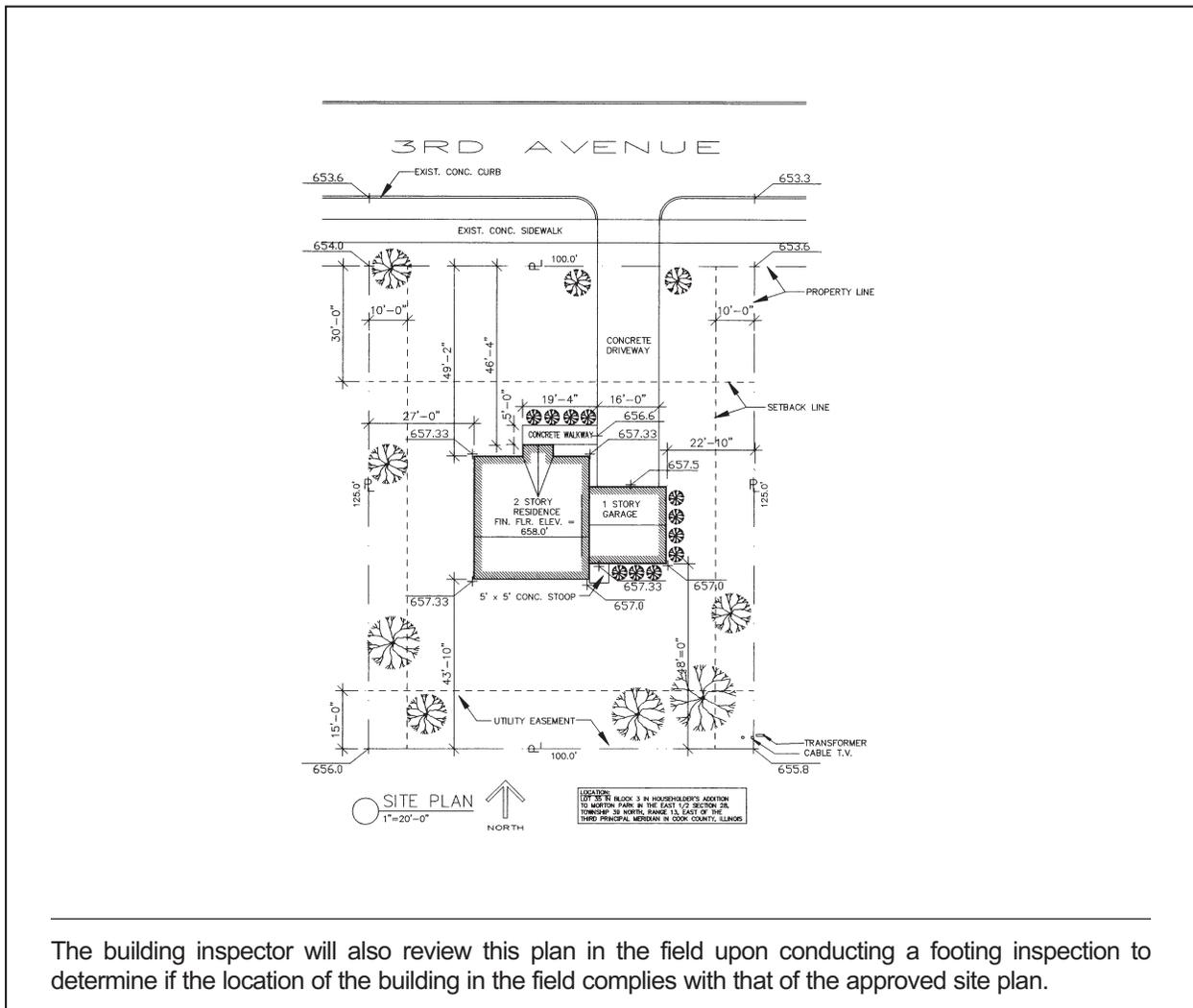
The building inspector will also review this plan in the field upon conducting a footing inspection to determine if the location of the building in the field complies with that of the approved site plan.
