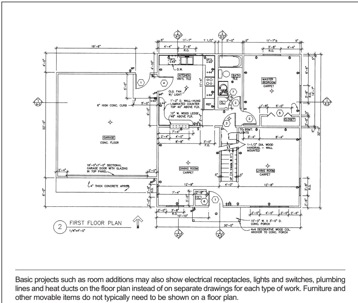
Basic projects such as room additions may also show electrical receptacles, lights and switches, plumbing lines and heat ducts on the floor plan instead of on separate drawings for each type of work. Furniture and other movable items do not typically need to be shown on a floor plan.
