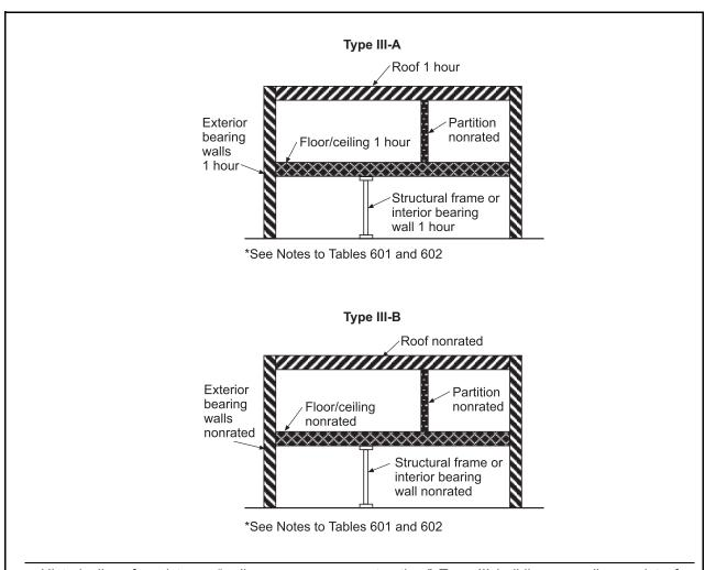
Historically referred to as "ordinary masonry construction," Type III buildings usually consist of concrete or masonry exterior walls with wood floor and roof systems. However, the SBC 201 permits such walls to contain fire-retardant-treated wood as an element of the exterior wall construction.
