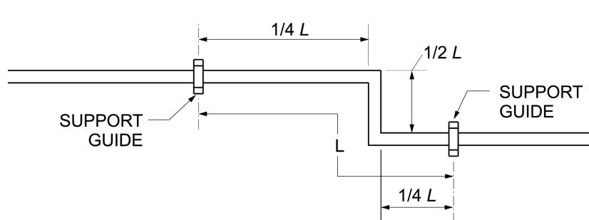
OFFSET PIPING MUST BE SUPPORTED WITH HANGERS, SLIDE PLATES OR SPRING HANGERS.
