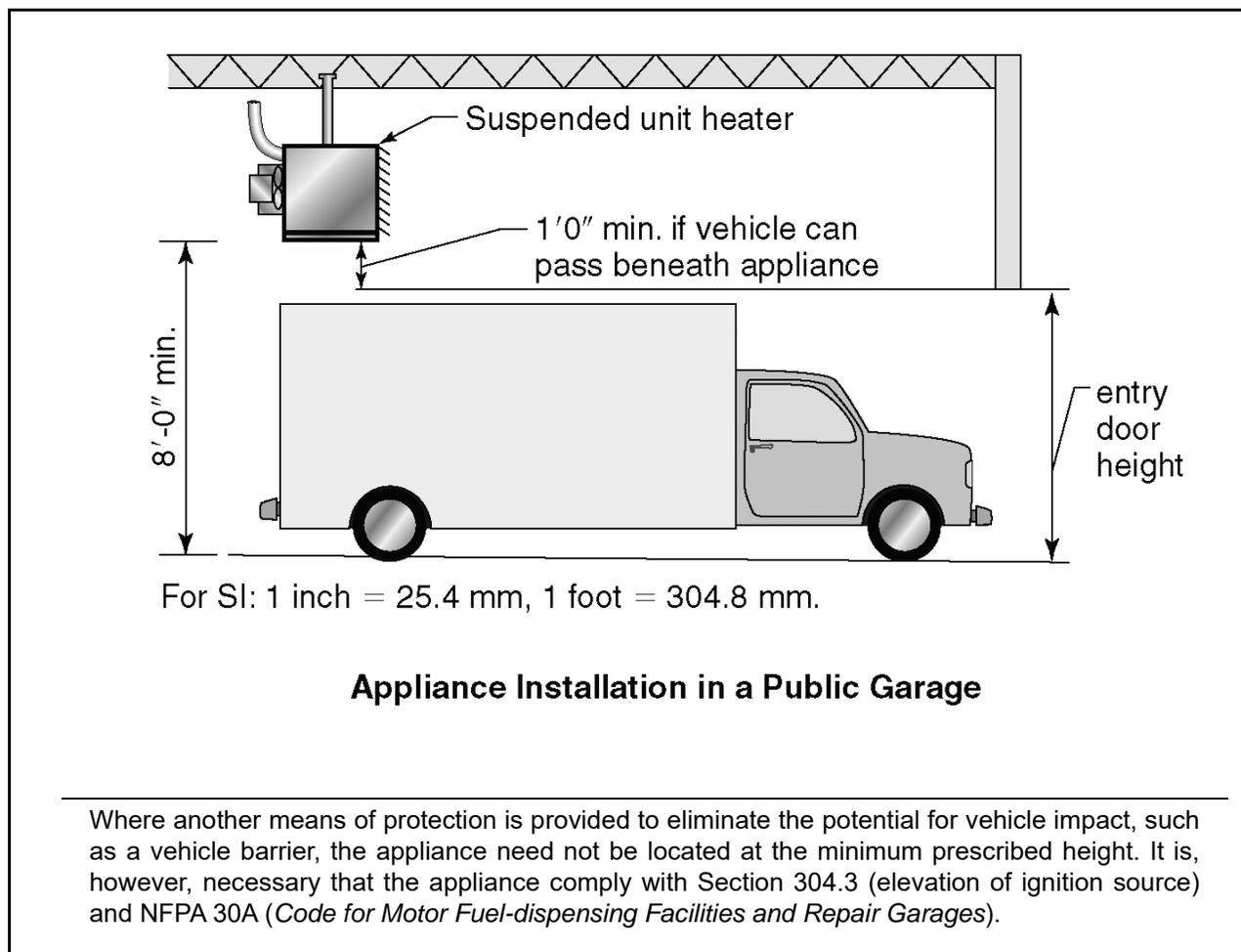
**Code Text:** *Appliances located in private garages and carports shall be installed with a minimum clearance of 6 feet (1829 mm) above the floor. See the exception addressing appliances that are protected from motor vehicle impact and installed in accordance with Section 304.3 (elevation of ignition source).*
