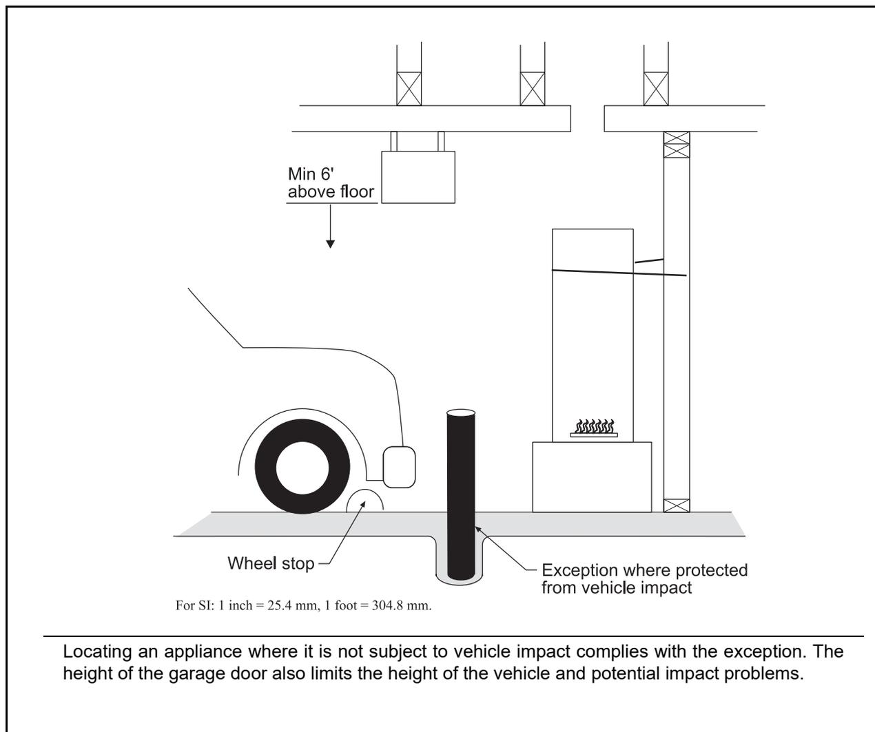
**Code Text:** *Equipment and appliances installed at grade level shall be supported on a level concrete slab or other approved material extending not less than 3 inches (76 mm) above adjoining grade or shall be suspended not less than 6 inches (152 mm) above adjoining grade.*
