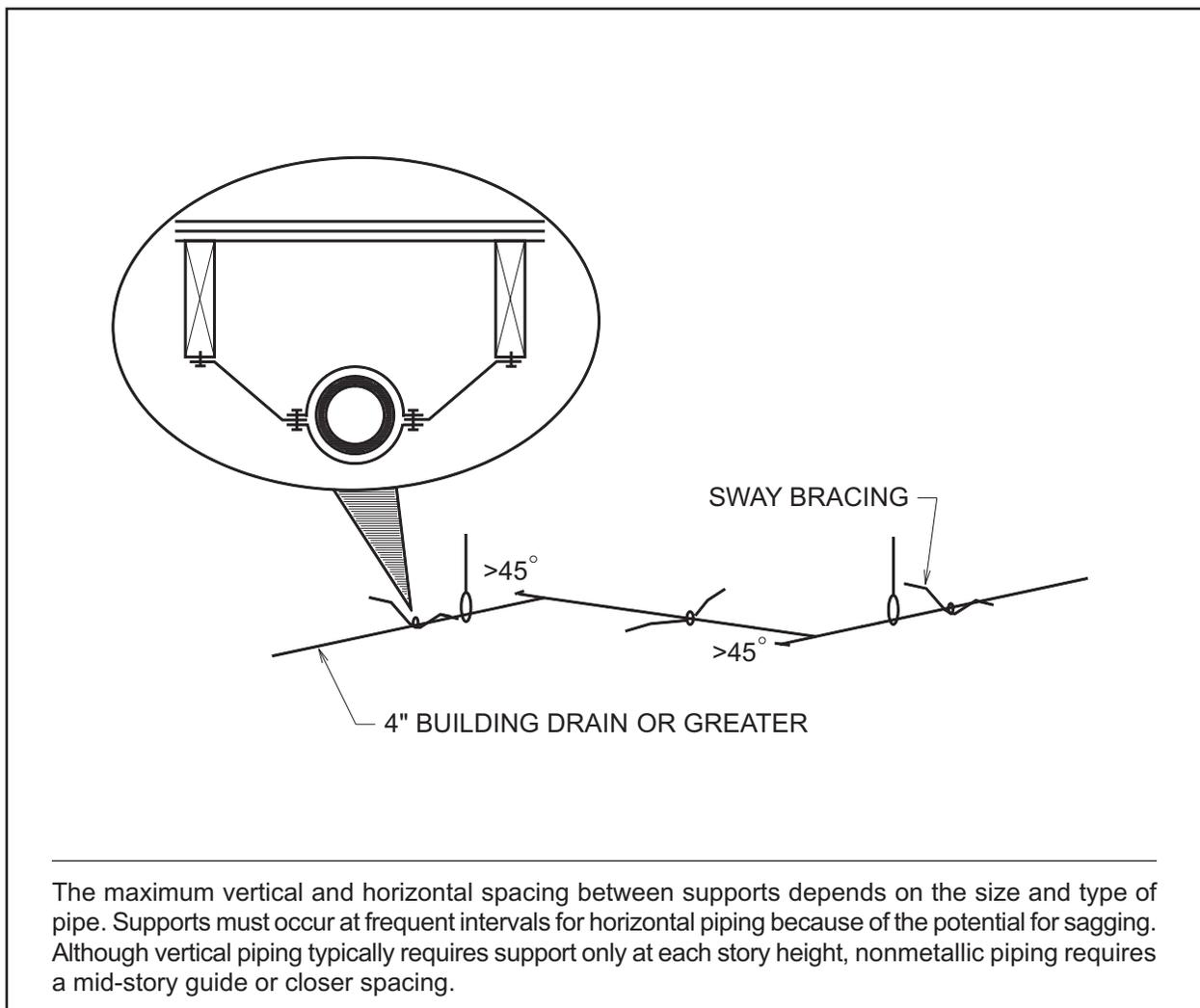
**Code Text:** *Anchorage shall be provided to restrain drainage piping from axial movement. For pipe sizes greater than 4 inches (102 mm), restraints shall be provided for drain pipes at all changes in direction and at all changes in diameter greater than two pipe sizes. Braces, blocks, rodding and other suitable methods as specified by the coupling manufacturer shall be utilized.*
