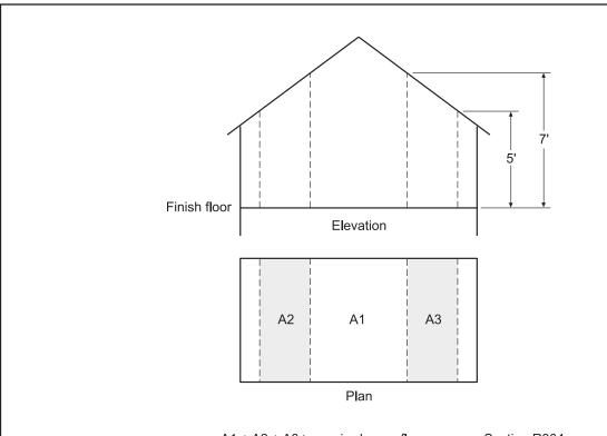
A1 + A2 + A3 ≥ required room floor area per Section R304
