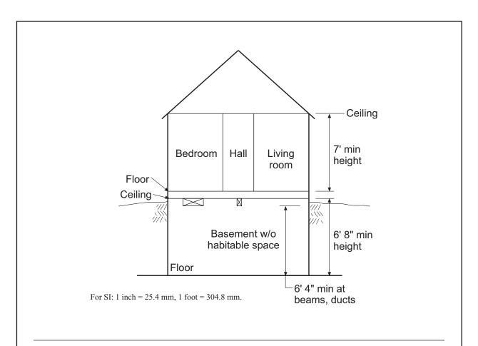
Three different minimum ceiling heights are applicable to basements. In habitable spaces and hallways, the minimum required height is 7 feet. Other areas of the basement only need a minimum ceiling height of 6 feet 8 inches. Where beams, ducts and other obstructions exist, a headroom clearance of 6 feet 4 inches is mandated.
