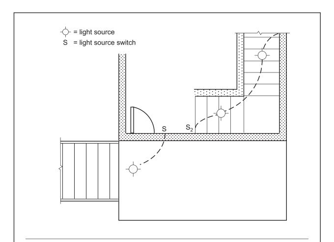
Unless the light sources are on continuously or automatically activated, interior stairway lights must be controlled from both the top and bottom of each stairway consisting of six or more risers. For exterior stairway lighting, the control switch is to be located within the dwelling unit.
