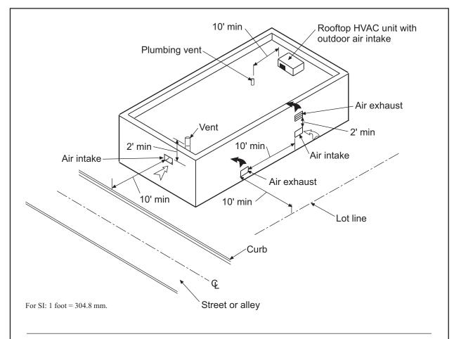
Outdoor air exhaust and intake openings are regulated in the same manner as other openings in exterior walls. As such, they are not permitted in walls having a fire separation distance of less than 3 feet, except in exterior walls that are perpendicular to the lot line.
